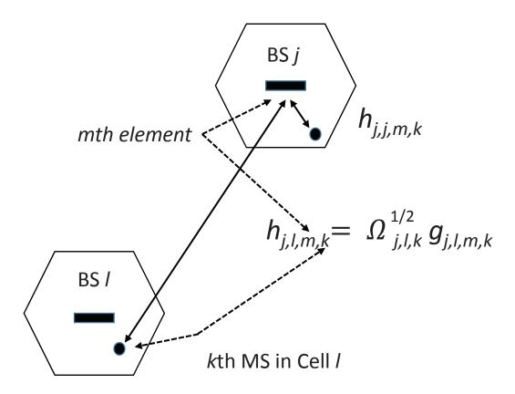
Propagation coefficient between kth MS in Cell  $\ell$  and the mth antenna element in Cell j.
