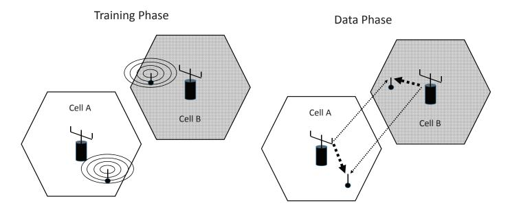
Pilot contamination in massive MIMO. During the pilot phase (left) the BS overhears the pilot transmissions from MSs in other cells. During the data phase (right) the BS partially beamforms to the MSs it has overhead in other cells
