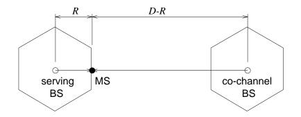
Worst case interference from a single co-channel base-station.
