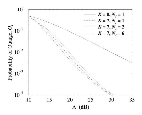
Probability of outage with multiple interferers. The desired signal is Ricean faded with various Rice factors, while the interfering signals are Rayleigh faded and of equal power;  $\lambda_{\rm th} = 10.0$  dB.
